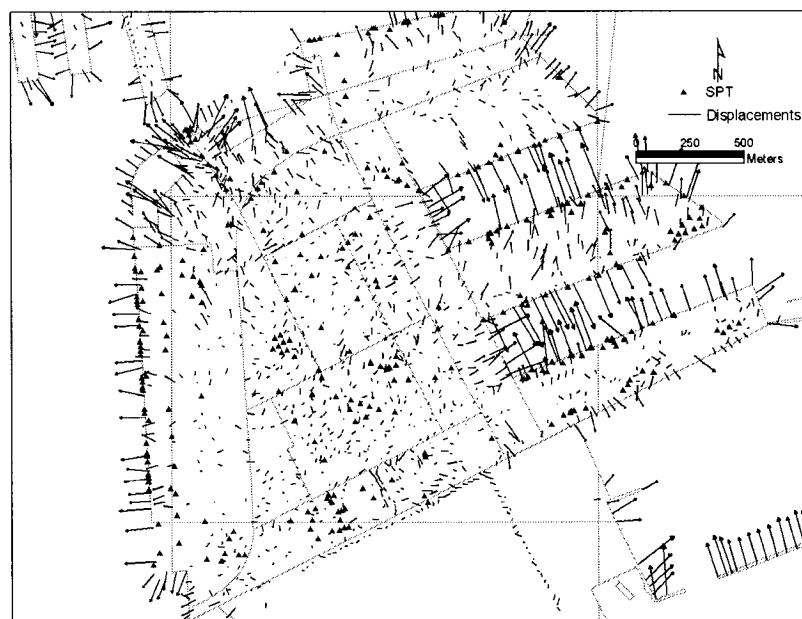
Figure 3-5. Displacement vector and borehole location in Port Island (data after Tanaka and Okimura, 2001).
