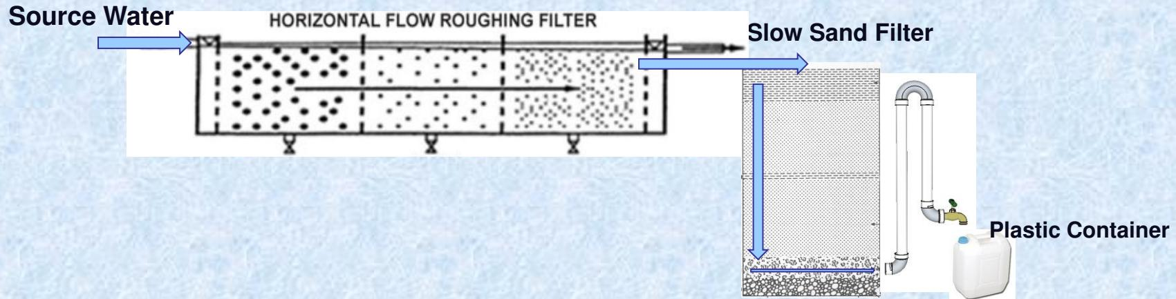
**Schematic of Main Components of Treatment Process**
