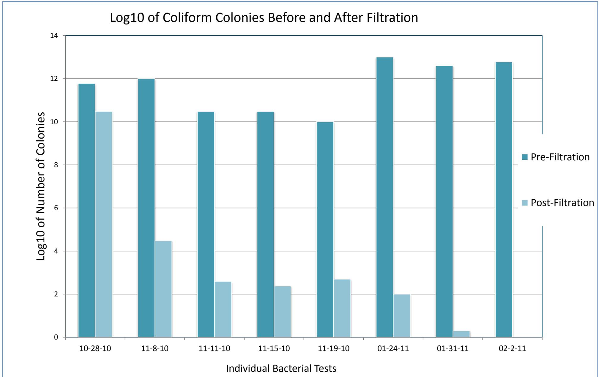
In the second phase of testing, coliform colony removal demonstrated higher removal efficiency over time, particularly after a periodic cleaning on January 20th. Even with extremely high concentrations of coliform and arsenic entering, the filter effectively removes over 99.999999%.
