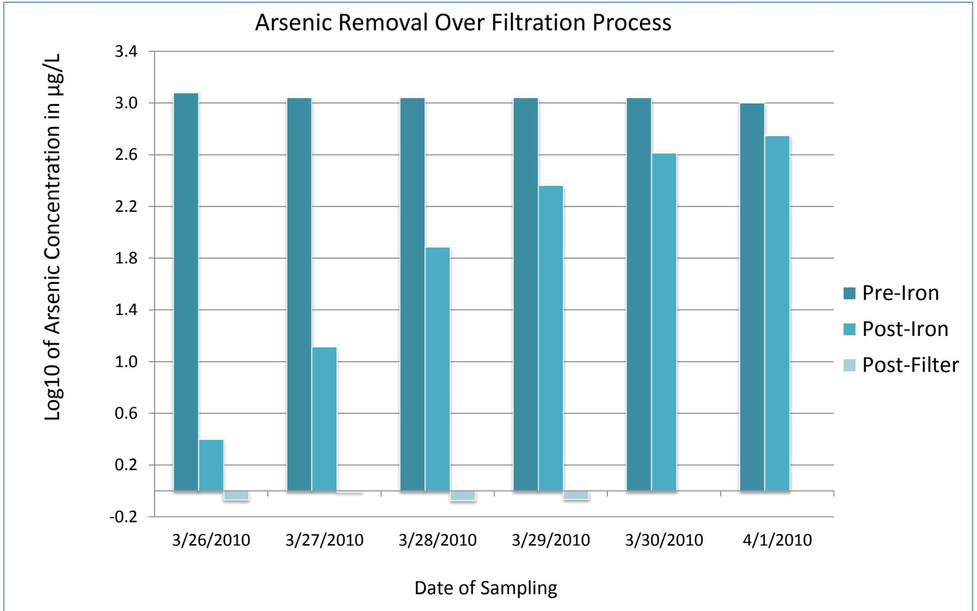
Test results show that the sand column was **initially** effective at removing arsenic, but quickly became saturated and almost completely ineffective. However, the biofilter removed nearly all arsenate from water regardless of the iron column's performance.
