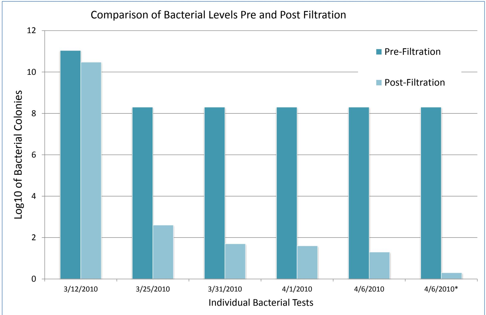
After a month of testing, the biofilter reduced bacterial concentrations by over 99.99%. Test results show the improvement of removal rates over the time period, reflecting the development of the schmutzdecke.
