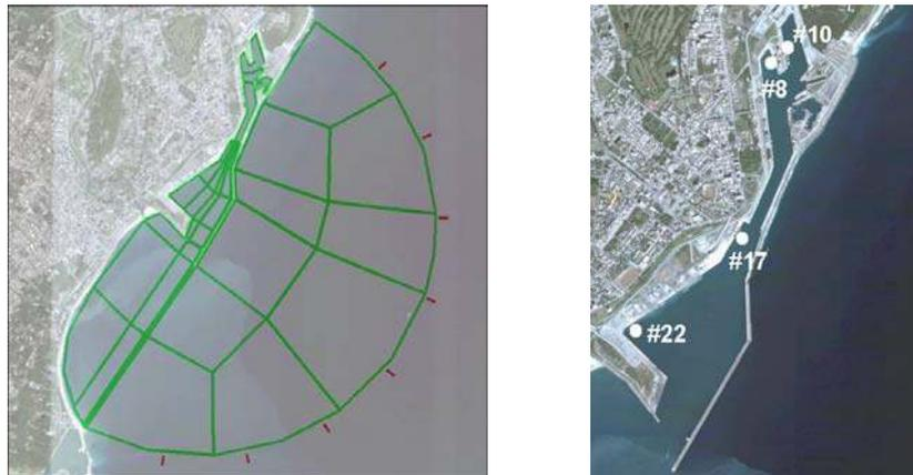
Figure 5.18 Air photos of Hualien Harbor, Taiwan with simulation domain imposed (left) and stations #8, #10, #17 and #22 indicated (right)
