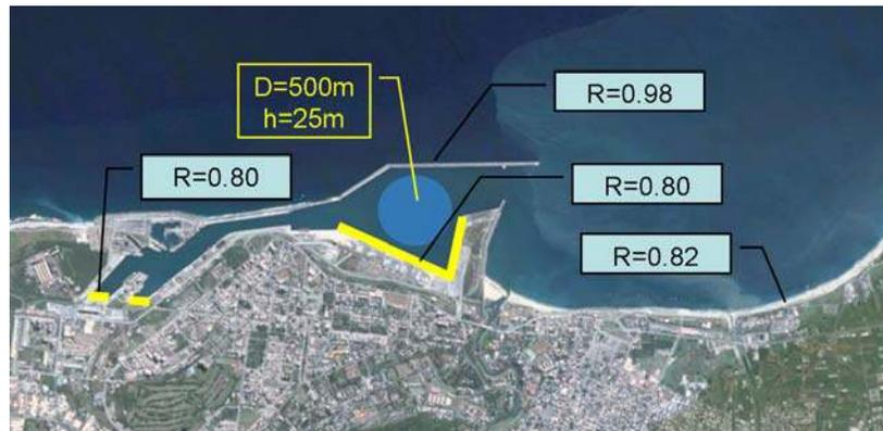
Figure 5.24 Layout of the energy dissipater modification strategy with reflection coefficients indicated
