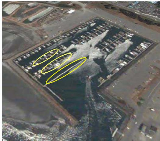
Figure 4.2 Air photo of the small inner harbor in Crescent City Harbor with the broken docks during the tsunami event on November 15, 2006 noted
