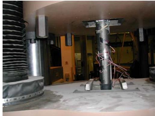
Figure 3.23: NMB splice sleeve test
