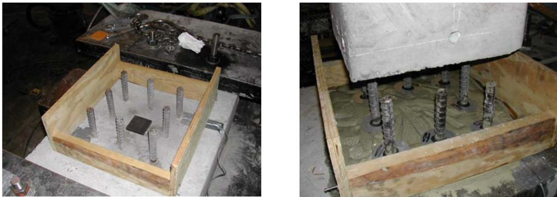
Figure 3.20: Column to footing connection
