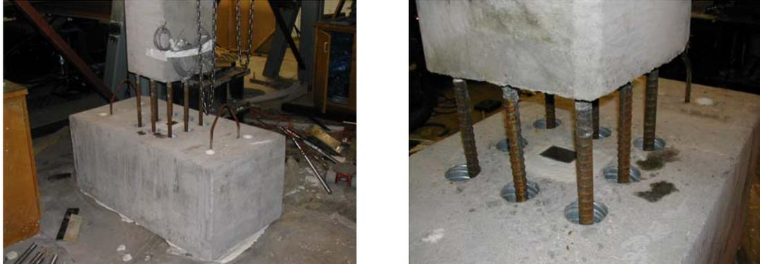
Figure 3.24: Column-footing connection of test model 2
