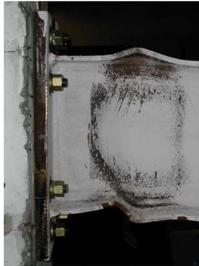
Figure 3.30: Buckling of steel beam RBS of TS1
