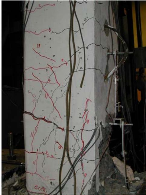
Figure 3.32: Cracking of column of TS1
