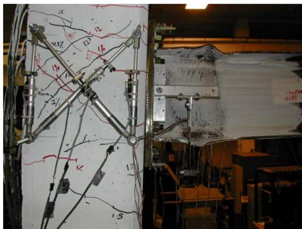
Figure 3.31: Cracking of beam-column joint of TS2
