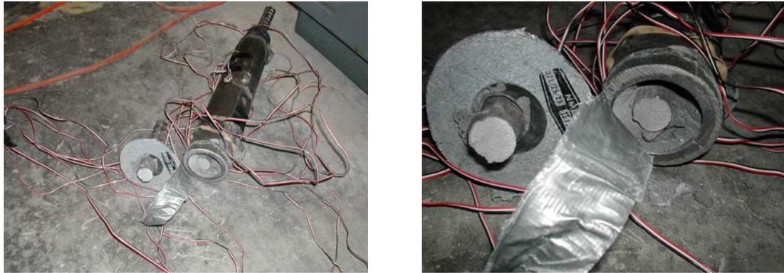
Figure C, continued: Failure of NMB Splice Sleeve Coupler
