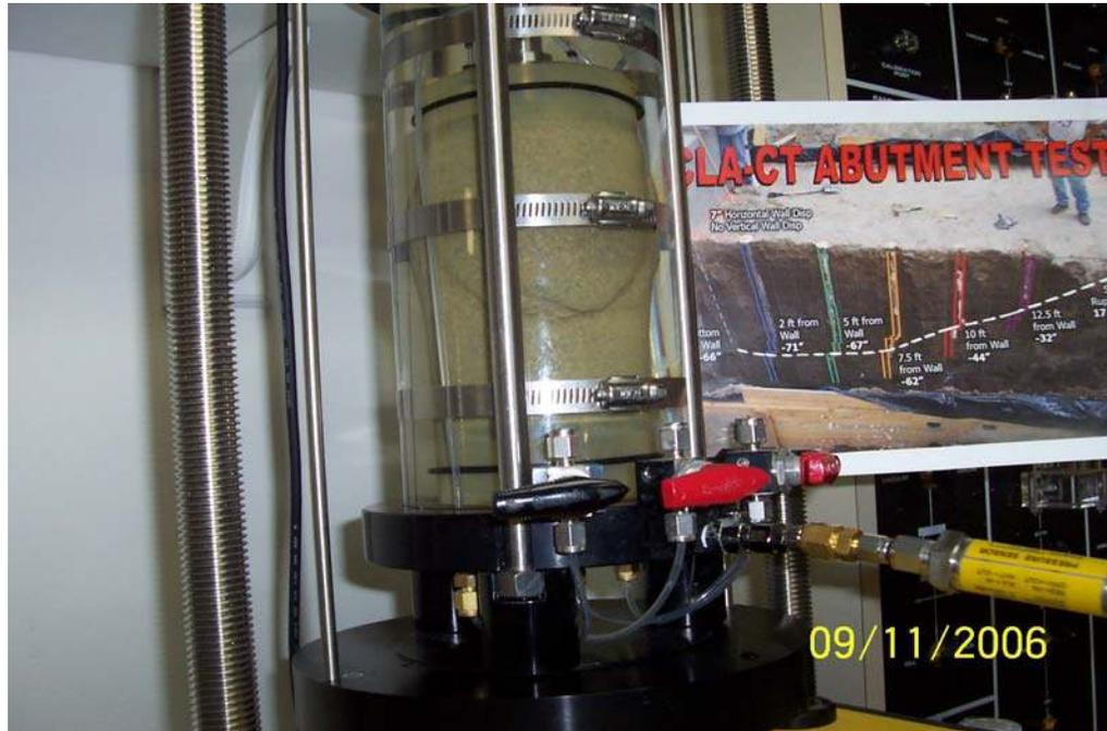
Figure 4.15: UCLA-CT Abutment Backfill Triaxial Test
