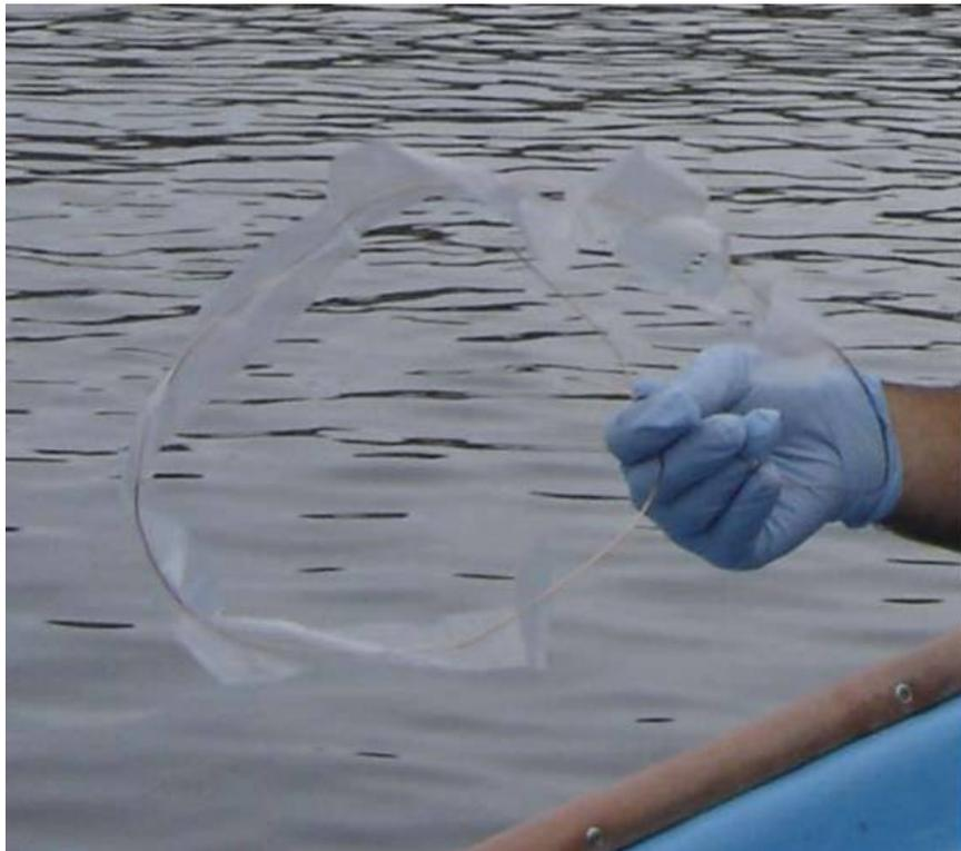
**Figure 2.5 A Polyethylene Device Ready for Field Deployment (Sayre 2006)**
