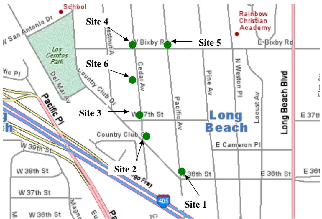
**Figure 4.4 Sampling Site Locations for Study 3: Virus Accumulation (Rand McNally and Company 2007). Site 5 was at a high point, and received flow only from adjacent homes.**
