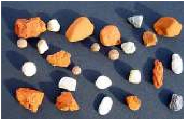
Figure 7-16 Variation of grains particle size and shape – important factors for packing density
