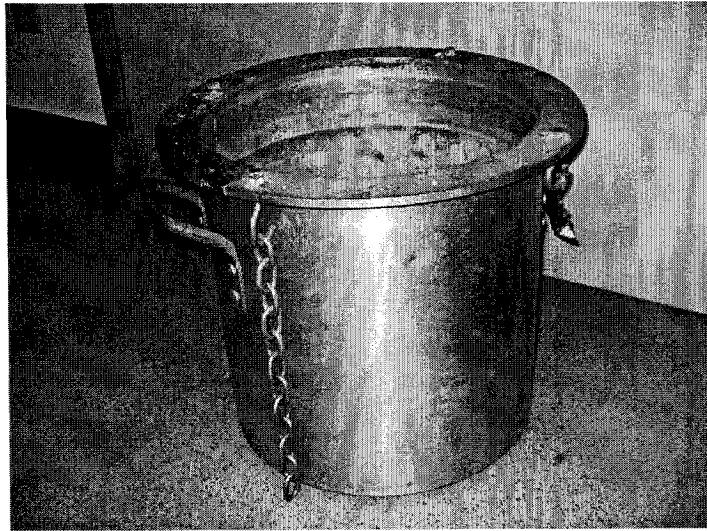
Figure 3-9. Cylindrical bucket used for centrifuge pile tests.
