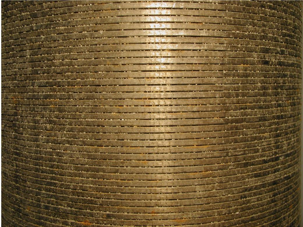
Photo A3.4 – 0.040 SSWWS After Testing With 20% Clogged
