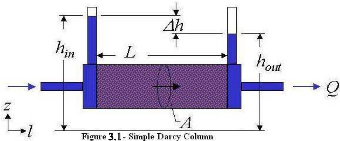
$Q$  = volumetric flow rate ( $m^3/s$  or  $ft^3/s$ ),  $A$  = flow area perpendicular to  $L$  ( $m^2$  or  $ft^2$ ),  $K$  = hydraulic conductivity ( $m/s$  or  $ft/s$ ),
