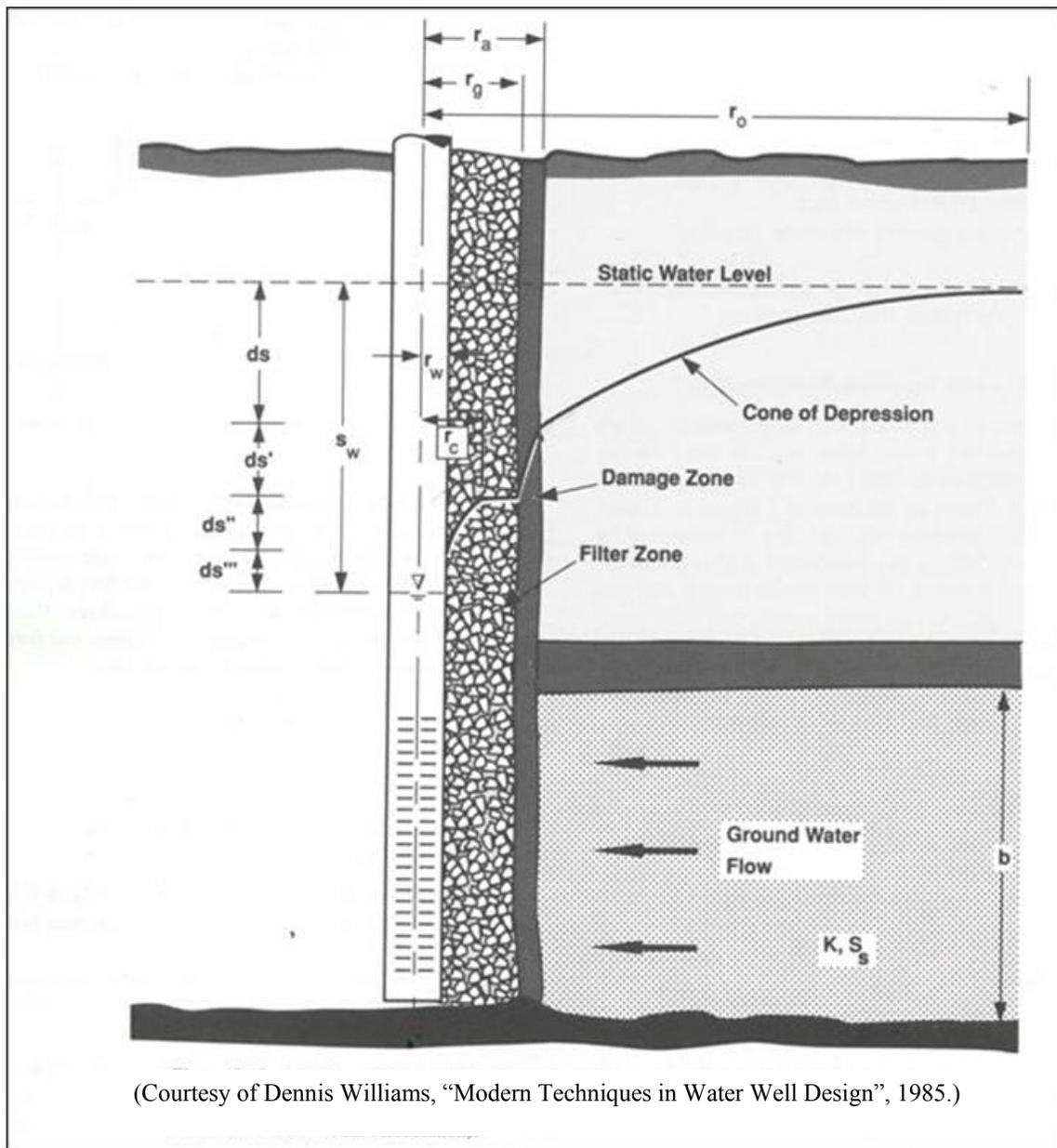
A figure of these losses in relation to a pumping well is seen in Figure 3.3. The formation or aquifer loss is the head loss or drawdown at the interface between the aquifer and the
