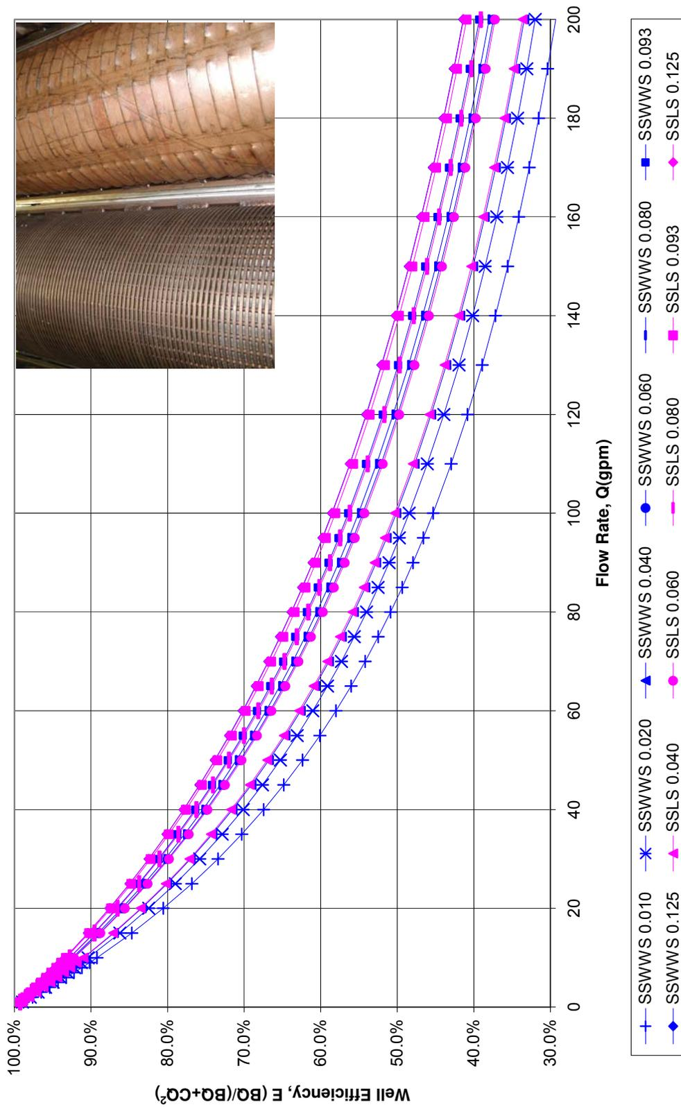
Figure 8.4 - 0.093 in. Slot Size vs. 0.080 in. Slot Size Well Efficiencies
