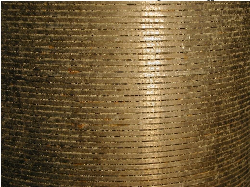
Photo A3.3 – 0.020 SSWWS After Testing With 75% Clogged
