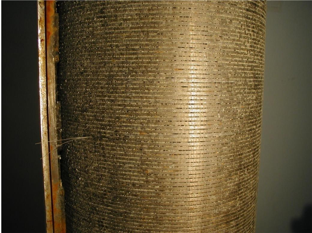
Photo A3.2 – 0.010 SSWWS After Testing With 85% Clogged
