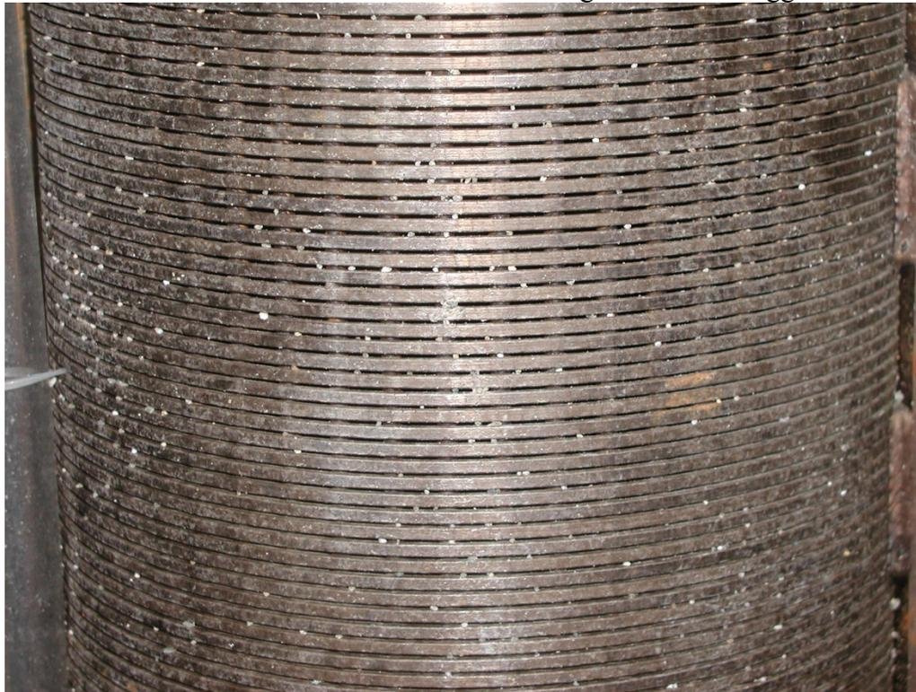
Photo A3.5 – 0.040 SSWWS After Testing
