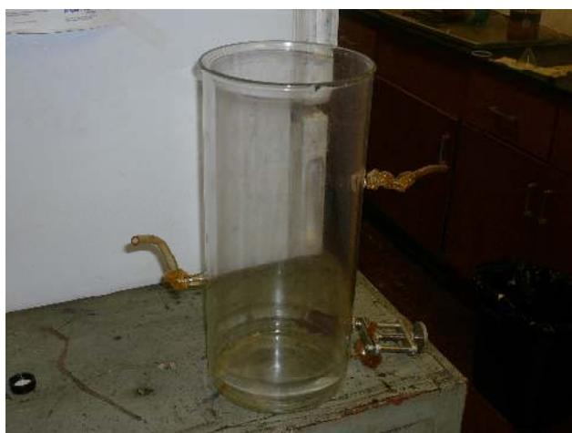
Figure 5.5 Photo of glass reactor
