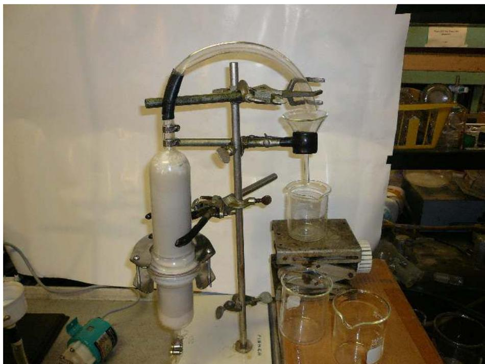
Figure 5.7 Fluidized bed reactor setup
