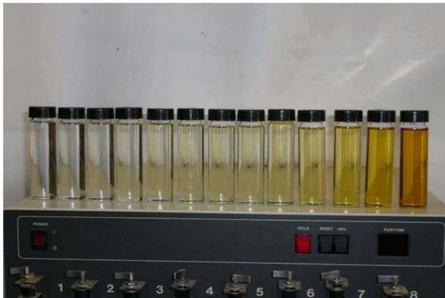
Figure 5.26 Color change of effluent due to saturation of adsorbent
