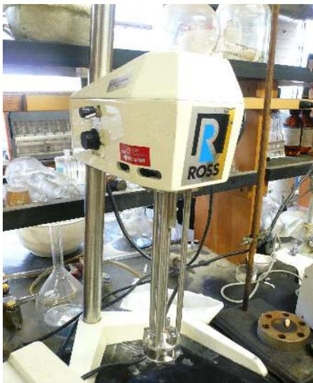
Figure 5.2 High shear mixer
