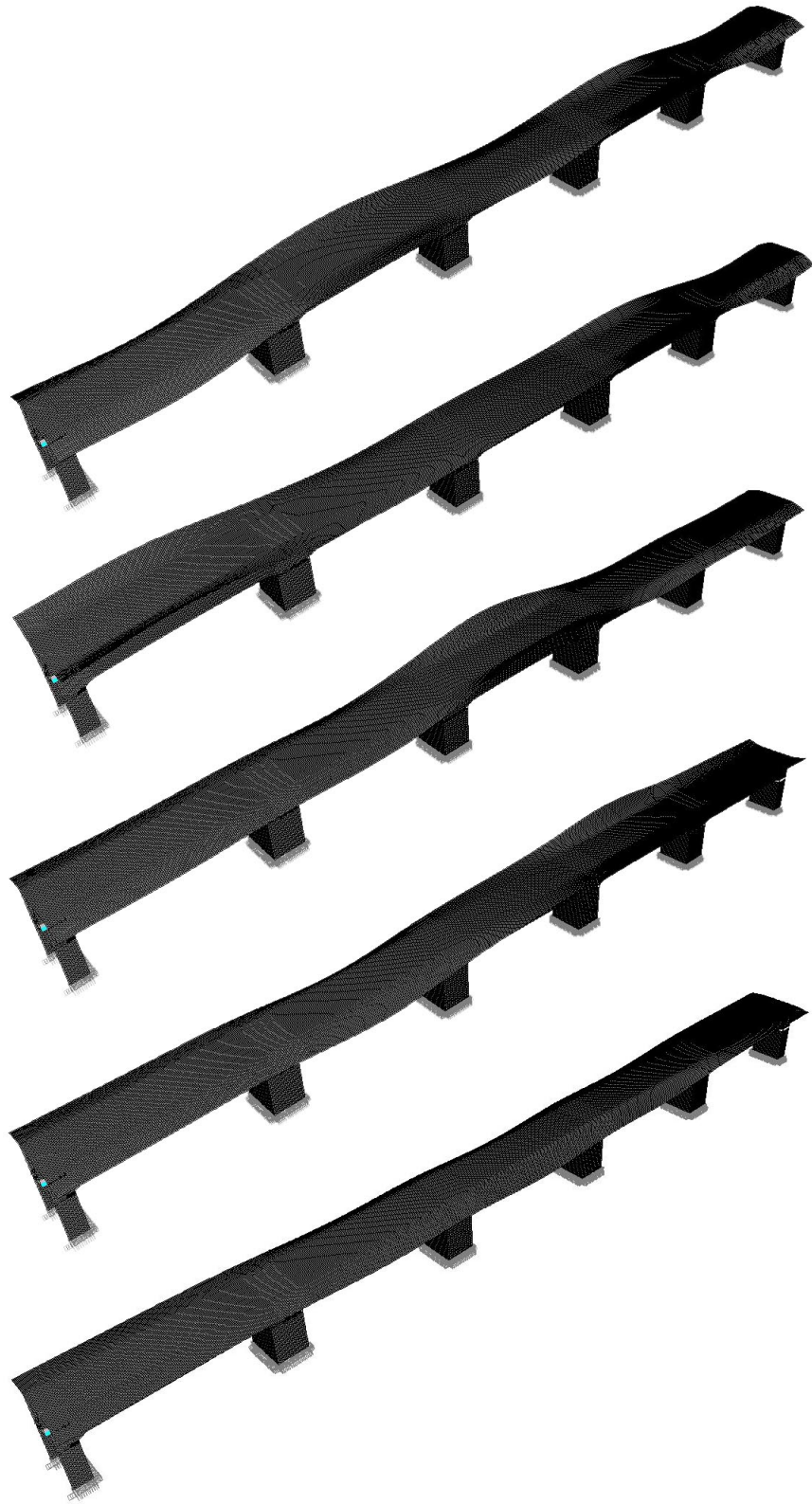
Figure 4.4 – Second Five Modes Shapes of a 5-span Finite Element Model.
