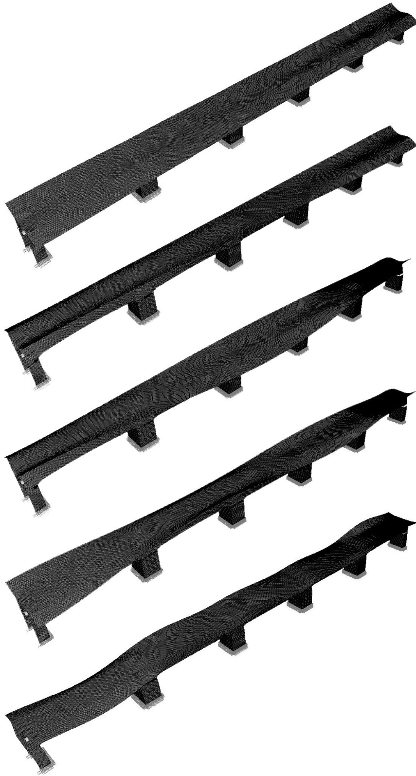
Figure 4.3 – First Five Modes Shapes of a 5-span Finite Element Model.
