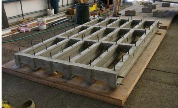
Figure 5.3: Pre-cast bridge specimen prior to attachment of deck ( Bradner and Cox (2008)).
