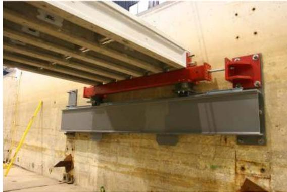
Figure 5.4: Test setup installed in Large Wave Flume ( Bradner and Cox (2008))
