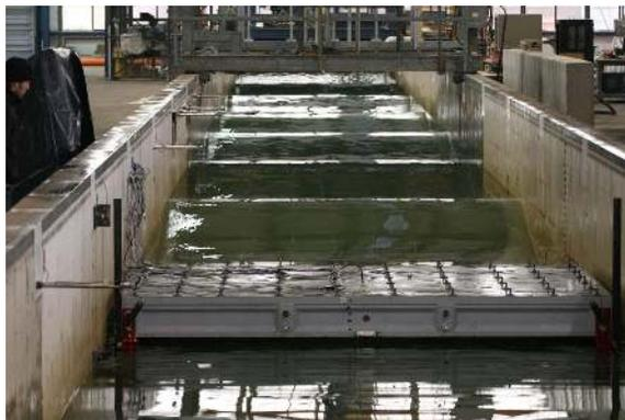
Figure 5.7: Photo of the bridge specimen during wave trial ( Bradner and Cox (2008)).
