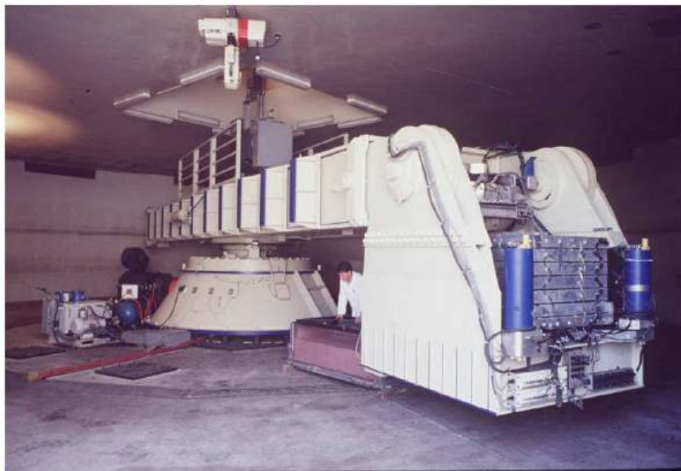
Figure 4-16: UC Davis Centrifuge (9.1 m radius and 240 g-tonnes)
